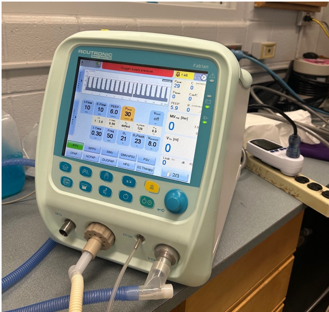
Figure 2.3.1 The Fabian™ HFO ventilator was connected to the RioRand Plug Power Meter Energy Monitor, where voltage was recorded. The “iPPV” mode was used with P_{\max} of 30 cmH 2 O, inspiratory time of 0.3 s, varying levels of PEEP, respiratory rate, and V_T .
