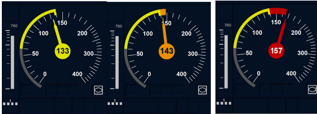
Figure A-10. ETCS level 1 speed and supervision information for target with braking needed (ERA, 2019)
