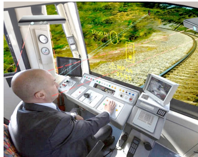
Figure A-16. An example of head up display (FRA, 2020)
