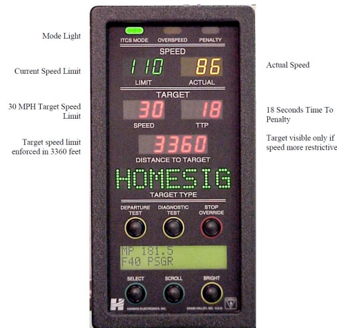
Figure A-5. ITCS in cab display (Roth and Multer, 2009)
