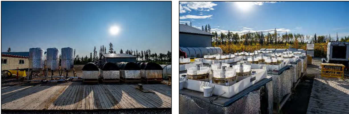
Figure 2 Mesocosm exposure tables, with and without shade cover. Holding tanks for treated OSPW and river water shown on left of first image.
