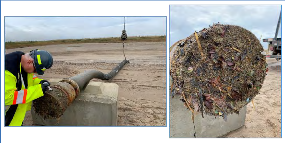
Figure 26: Fouling on the Screen of the Pump Intake (Stage 3)
