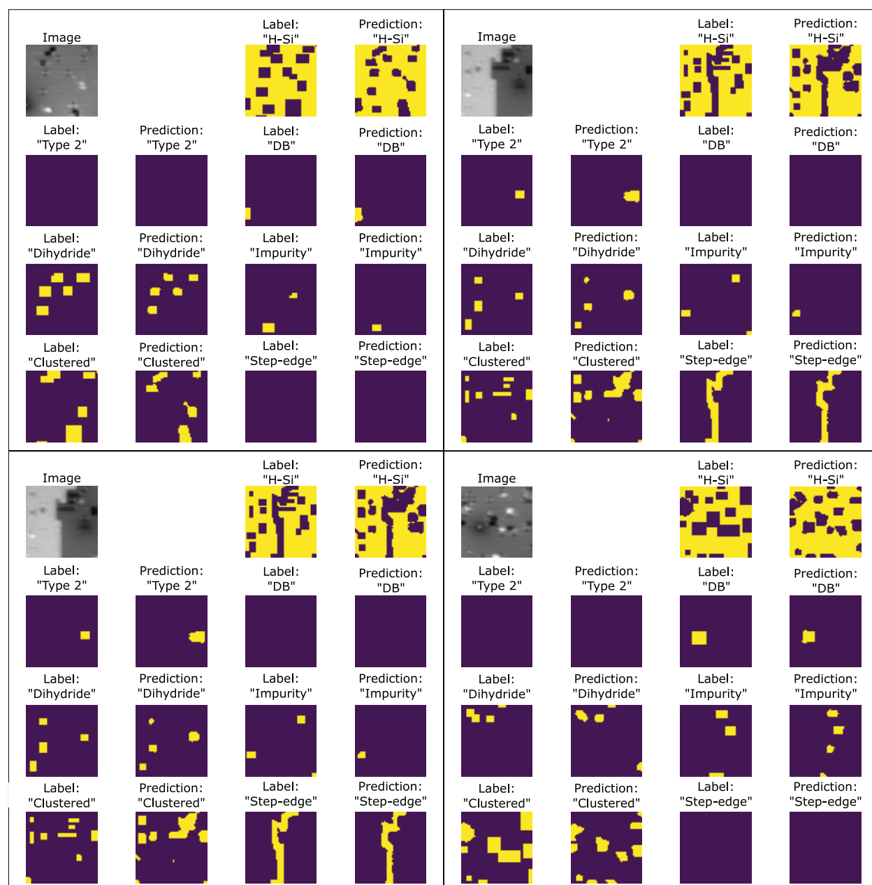
FIGURE 4.9: Heat maps from a random selection of the test data set. True pixels are yellow while false pixels are purple. Each image is 12.5 \times 12.5 \text{ nm}^2 .
