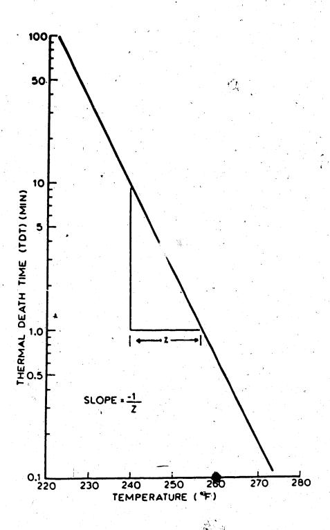
Figure 1.5 Thermal death time (TDT curve) for Clostridium botulinum in phosphate buffer. Source: Lund (1975).
