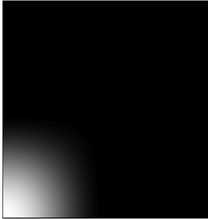
Figure 7: Tensor product of the ideal high-pass filter with itself in frequency domain (magnitude)
