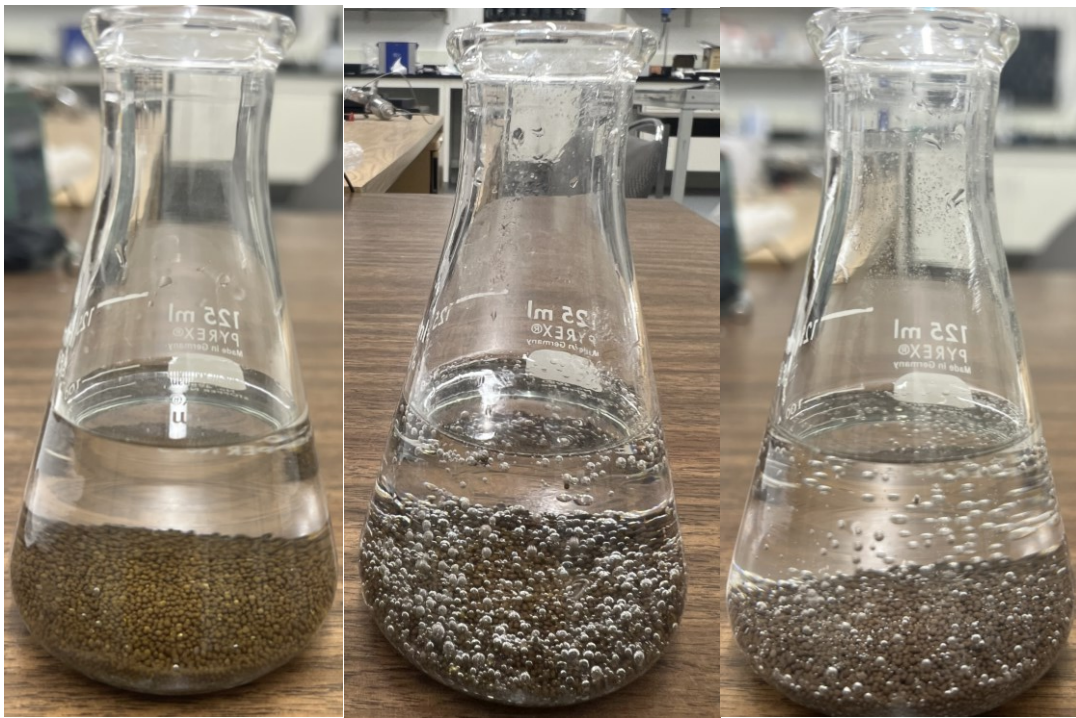
(a) (b) (c) Figure 2.17 Comparison of the interaction between air/CO 2 and different proppants: (a) Resin-coated proppants with air; (b) Resin-coated proppants with CO 2 ; (c) Ceramic proppants with CO 2
