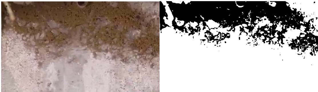
Figure 2.7 Distribution of resin-coated proppants with a mesh size of 30/50 in the investigated zone in the 4 mm wide fracture. The image is captured post the injection of acid with the rate of 21 ml/min to the fracturing fluid with 8 wt% of sodium bicarbonate. The left image is the original image, while the right one is the processed image. The proppant coverage ratio is measured to be 0.28262.
