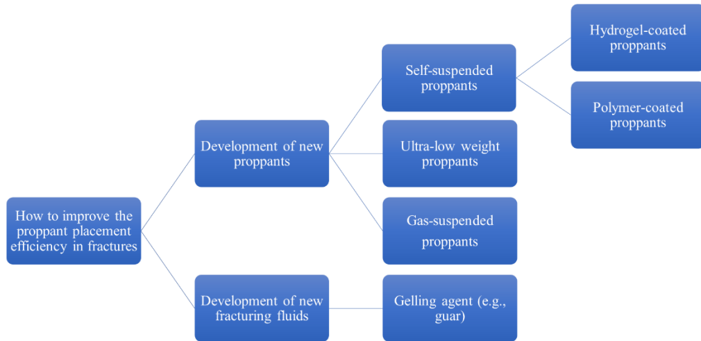
Figure 1.1 Summary of different approaches developed in the past to increase the proppant placement efficiency in fractures
