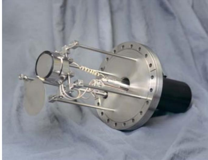
**Fig. 3.1.3.** PLD heater manufactured by Neocera Inc. [44].
