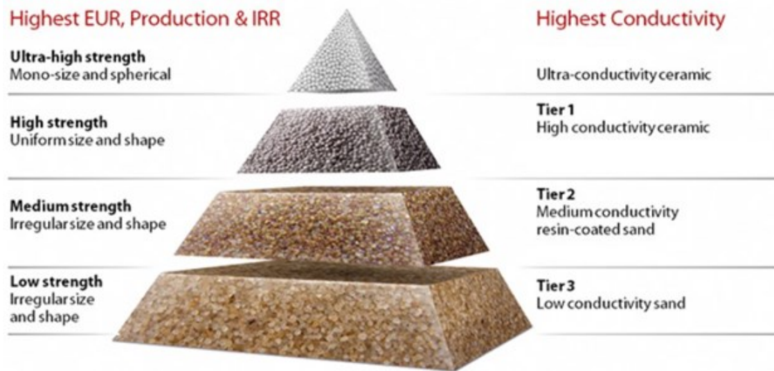
Figure 1.8: Four types of proppants commonly used in hydraulic fracturing (from ASD Report, 2015).
