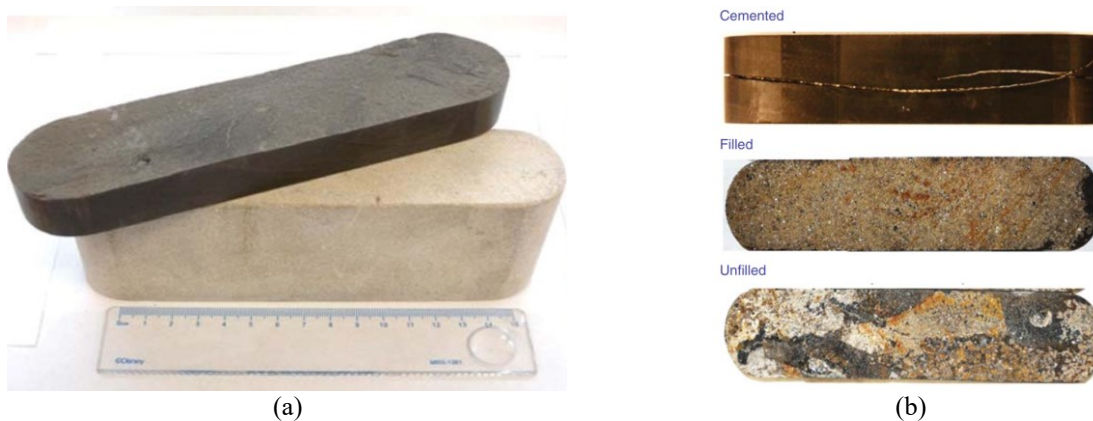
Figure G.1: (a) Dimensions of the shale samples used in the fracture conductivity measurements; (b) Three types of preserved natural fractures in the shale samples: cemented, filled and unfilled (from Zhang et al., 2014).
