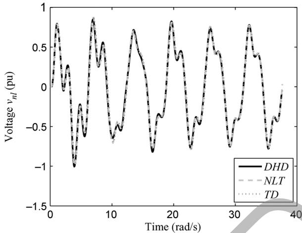
Fig. 9. Voltage across nonlinear load using the DHD, NLT hybrid, and the TD.
