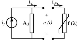
Fig. 2. Steady-state approach: Norton equivalent decomposition into linear and nonlinear subsystems.
