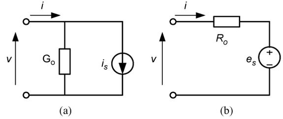
Fig. 1. Norton and Thevenin equivalents circuits for the  $z$  transform.
