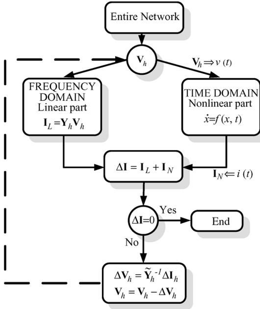
Fig. 3. Harmonic Balance Type B procedure.
