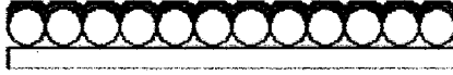
Figure 3.1: Experimental Samples: an array of silica microspheres on a substrate with a layer of Si nanocrystals on top. Drawing is not to scale.
