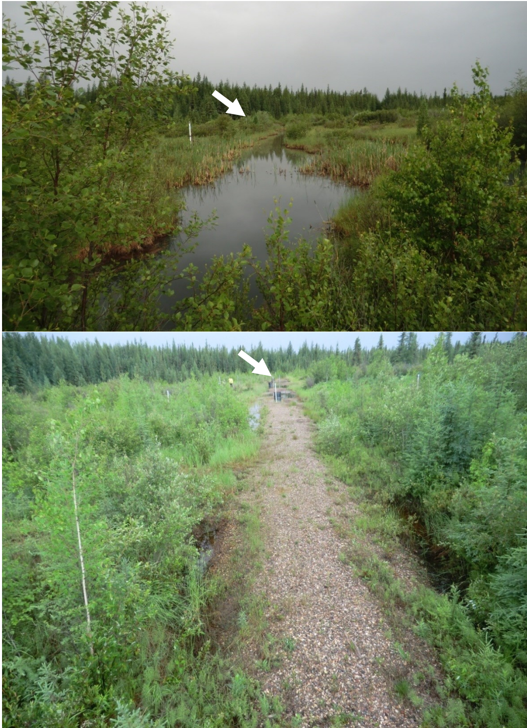
Figure 4.2 Photos of the two PRBs. Top: The partially water logged 2006 PRB (PRB2). Bottom: The drier 2007 PRB (PRB1). Arrows point to the locations of wells 5 (top) and 15 (bottom), respectively.
