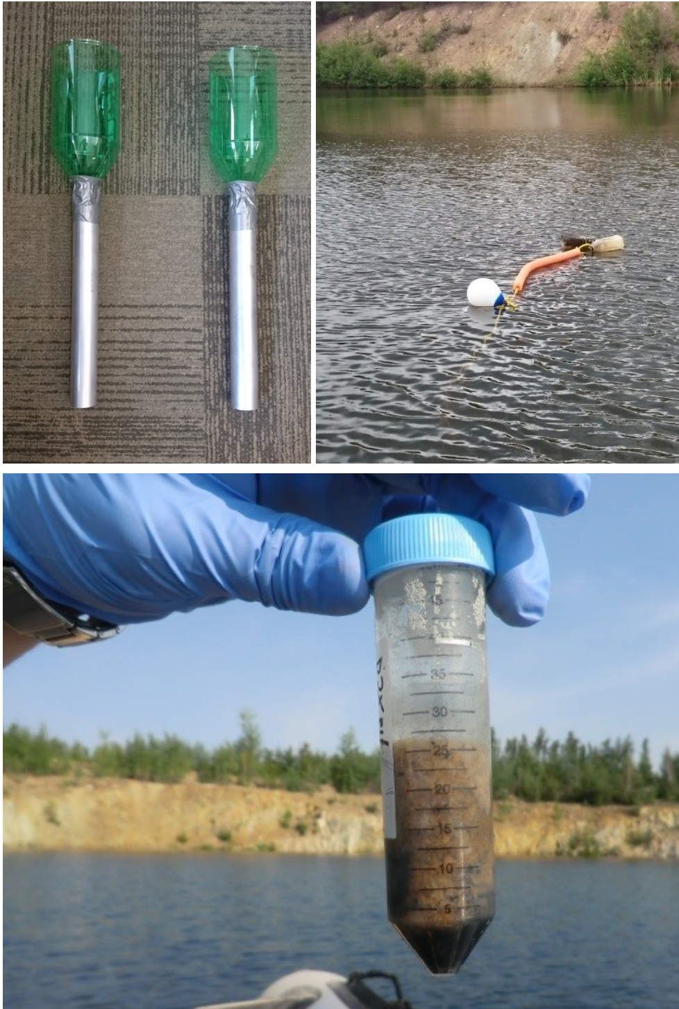
Figure B.10 Example photos of the sediment traps. Top left: two sediment traps with the aluminum pipes attached; the collection tube is inside the pipe; the funnel on top, made of a cut PET bottle had a surface area of 95 cm 2 . Top right: sediment trap after deployment in the D-pit in June 2017. The white buoy is carrying the sediment trap below; the plastic water log is keeping the white buoy at a distance to the center buoy. Bottom: collected sediments from the sediment trap retrieved from the DJX-pit in June 2018 after removing the funnel and after sealing the tube.
