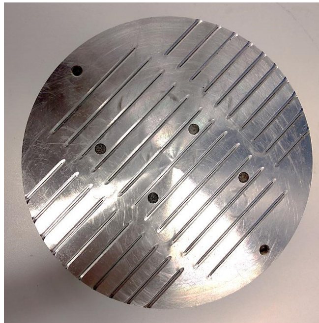
Figure 5-3. Multi-slot coupon with seamed slots
