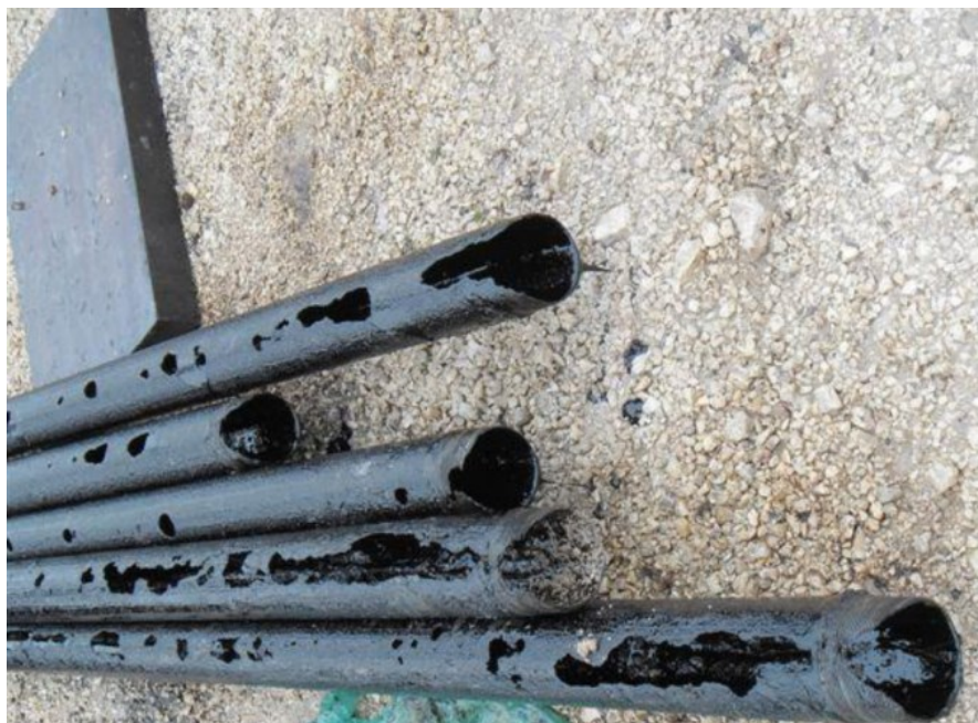
Figure 2-5. Liner damage after four years of production (After Hallman et al. 2015)
