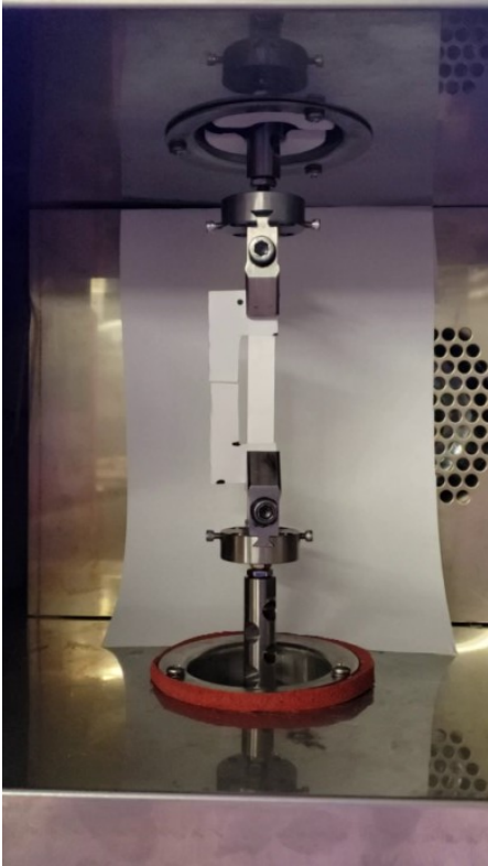
Figure 2-3 Rectangular sample of electrosun PCL/gelatin prepared for tensile test
