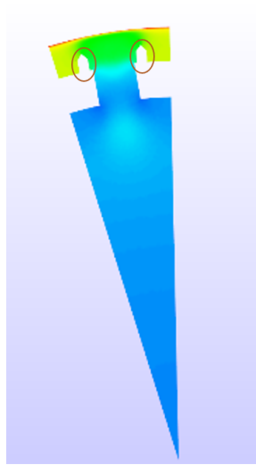
Figure 3.11: Stagnation zones at the rib wire locations.
