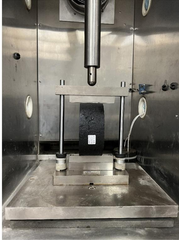
**Figure 4-6. IDEAL-CT test setup**
