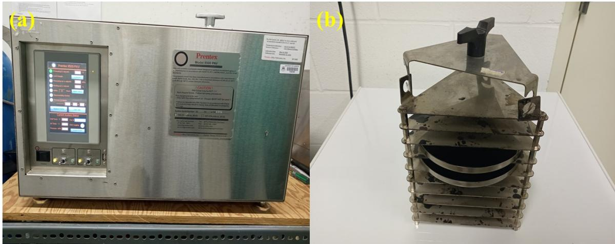
**Figure 2-4.** (a) Pressure aging vessel (PAV), (b) Binder samples in a PAV rack
