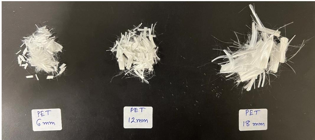
**Figure 4-3.** Polyethylene Terephthalate (PET) fibres in different lengths (from left to right: 6-mm, 12-mm, and 18-mm)
