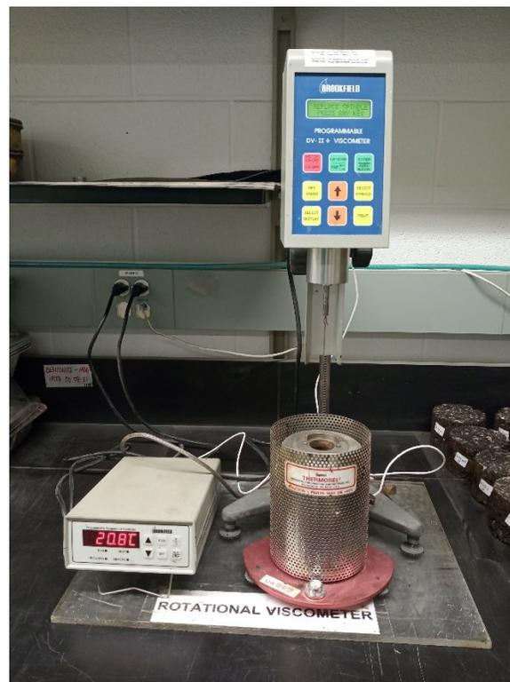
**Figure 2-7.** A rotational viscometer (RV)
