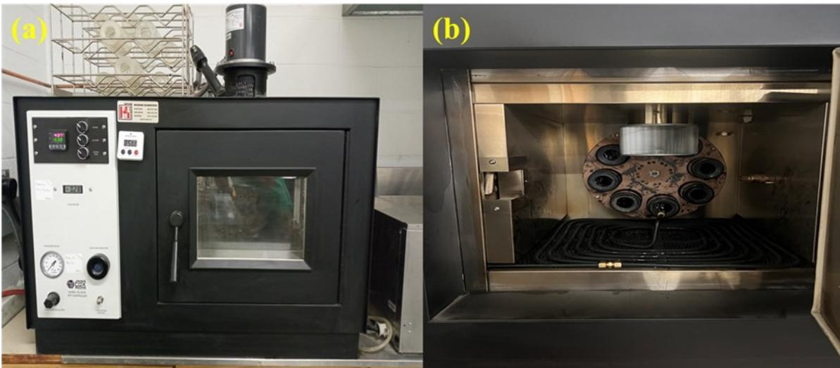
**Figure 2-3.** (a) Rolling thin film oven (RTFO), (b) RTFO carriage inside the oven
