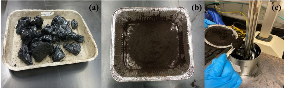
**Figure 4-2.** Asphaltenes (a) Solid form, (b) Powder form, (c) Binder modification using a high shear mixer
