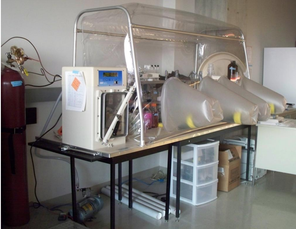
Figure 4-1: Anaerobic chamber to isolate the soil samples from an aerobic atmosphere.
