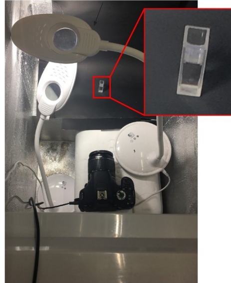
inside the freezer: lights, camera, and cuvette
