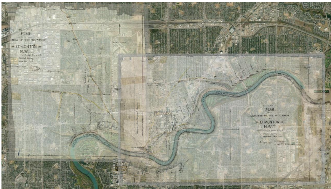
Figure 5.6: Georectification results of sheets one and two of 1878 King survey overlaying "World Imagery" basemap with both survey sheets at 50% transparency
