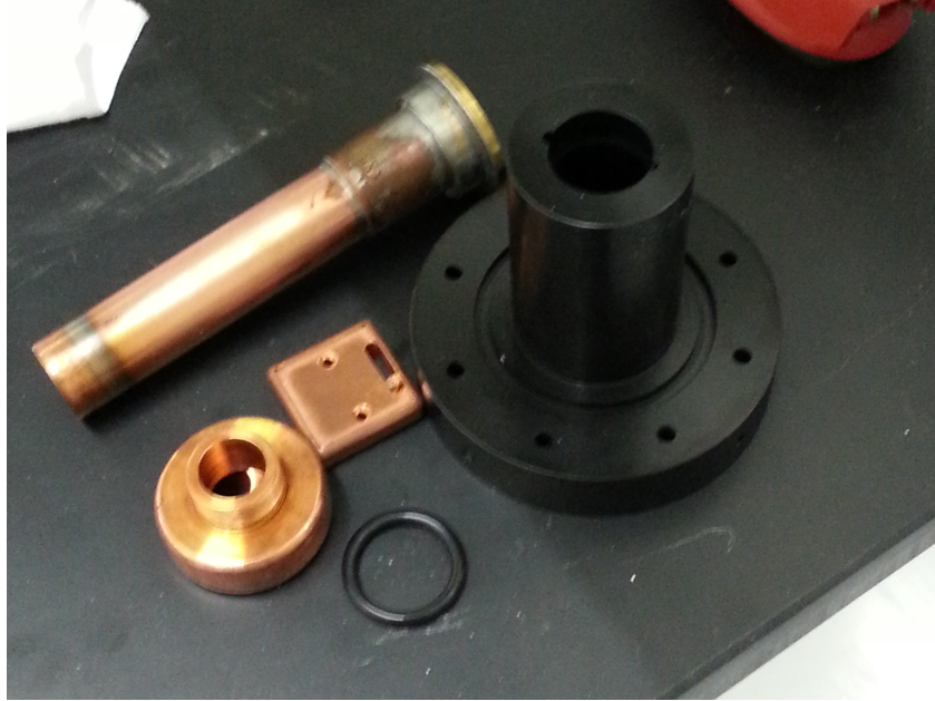
Figure 4.23: The feedthrough components that were tested as possible radon emitters.
