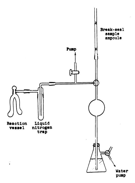
Apparatus for Preparation of Nitrogen Samples for
