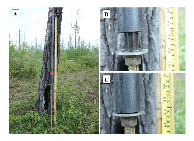
Appendix 9: Soil penetrometer developed for this thesis and used to measure soil resistance and strength (description in section: Field methods). Penetrometer body constructed of 2 m length, 1.5" schedule 40 steel pipe, and 1 m length penetration pin constructed of 1" solid steel (A). A sliding weight (7 kg) was dropped from 1.5 m height onto the collar of the penetration pin (B & C). A tape measure fixed to a stake was used to measure penetration depth to the nearest 0.5 cm.
