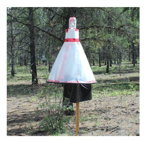
Appendix 6: Tabanid trap developed for this thesis based on design of Thorsteinson et al. (1965). Traps were designed to catch flies from the family Tabanidae (description in section: Field methods). Appendix 7: Correlation matrix of measured soil properties for 180 soil moisture and bulk density samples and 756 penetration depth measures taken in 4 land-cover types (marsh, deciduous, pine, and esker) in the summer of 2016 near Ronald Lake, Alberta.
