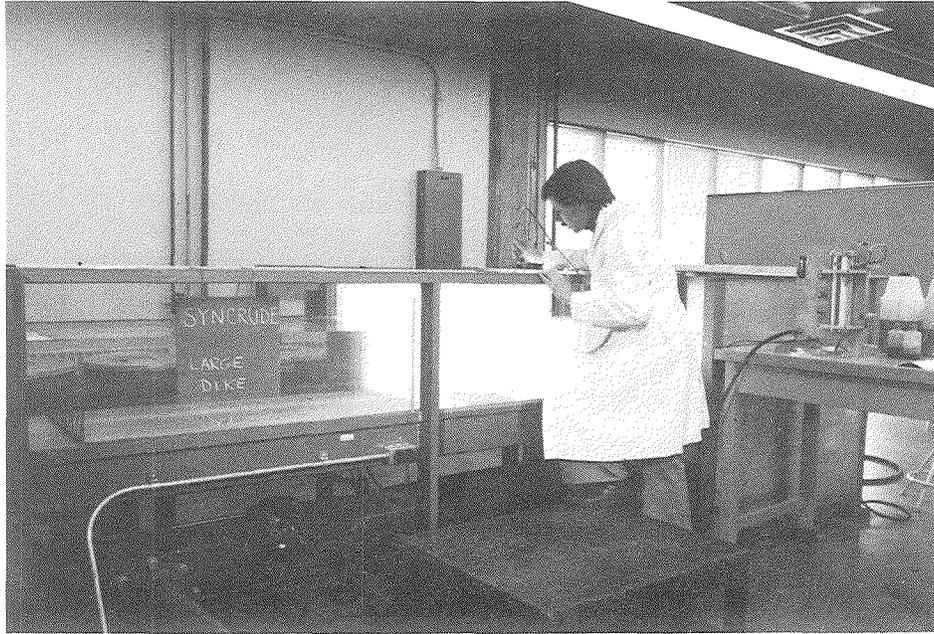
Figure 3-1. Water Channel and Dye Injector for Flow Visualization
