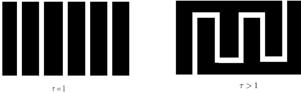
**Figure 1.5** – The tortuosity comparison of two porous media with same porosity
