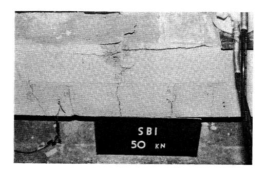
Plate 5.1 Failure of Beam SB1
