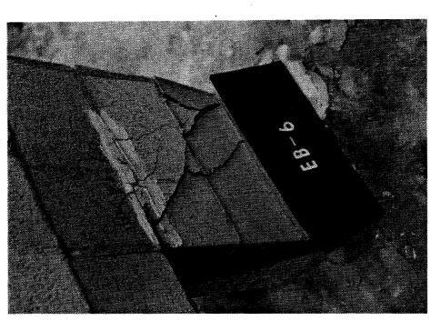
Plate 5.28 South Supporting Wall of Beam EB6 after Test
