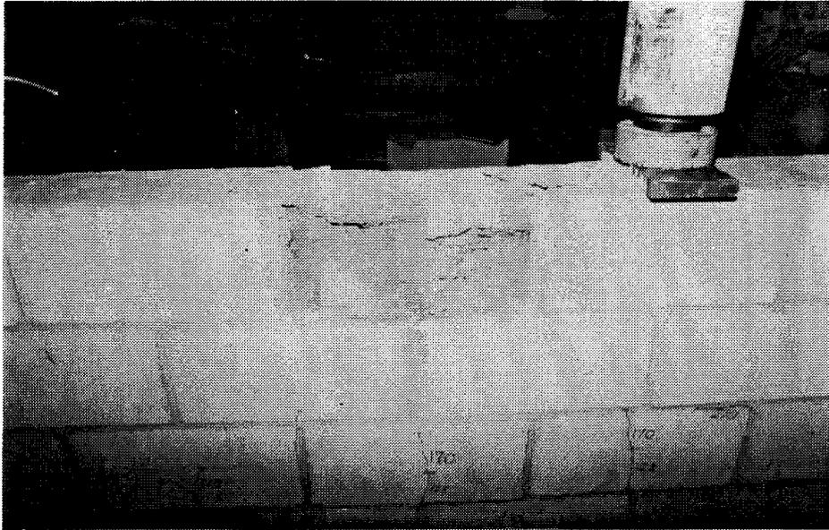
Plate 5.8 Failure of Beam RB2
