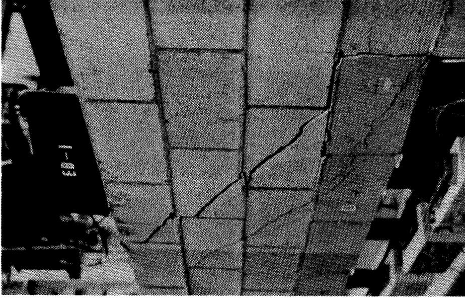
Plate 5.13 Failure of Beam EB1
