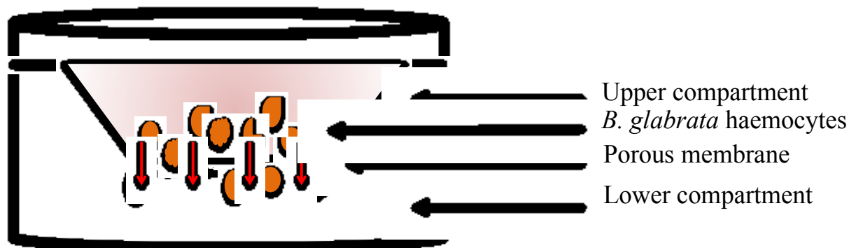
Figure 3.13 Chemotaxis apparatus set up
