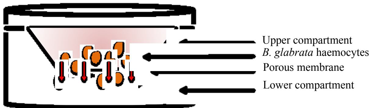
Figure 3.13 Chemotaxis apparatus set up
