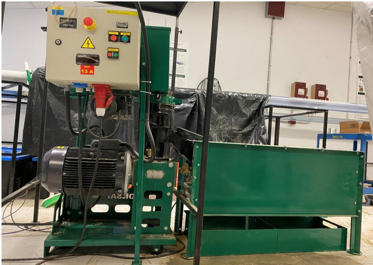
Figure 2.2. Pelletizer and screen assembly
