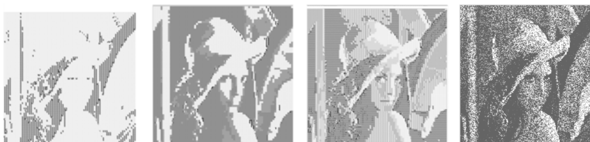
Figure 4.14: The progressive improvement of image quality using L^1 -norm stochastic VQ after 256, 512, 1024 and 2048 clock cycles.
