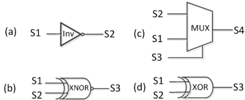
Figure 2.3: Stochastic arithmetic units in bipolar (signed) encoding: (a) S2 = -S1 ; (b) S3 = S1 \cdot S2 , ( S1 and S2 are uncorrelated sequences); (c) S4 = S3 \cdot S1 + (1 - S3) \cdot S2 ( S3 is a unipolar sequence); (d) S3 = -S1 \cdot S2 ( S1 and S2 are uncorrelated sequences).
