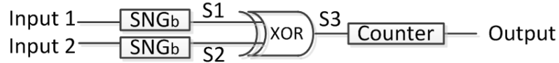
Figure C.2: Schematic of the stochastic absolute subtractor: S3 = |S1 - S2| ( S1 and S2 are correlated sequences).
