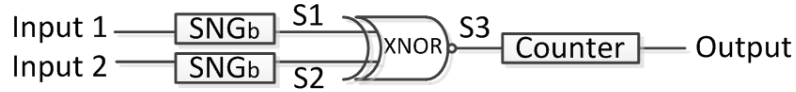
Figure 2.12: Schematic of the stochastic bipolar multiplier: S3 = S1 \cdot S2 ( S1 and S2 are uncorrelated bipolar sequences).
