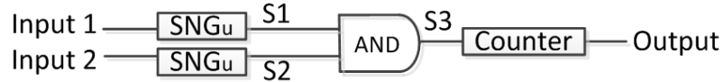
Figure 2.11: Schematic of the stochastic unipolar multiplier: S3 = S1 \cdot S2 ( S1 and S2 are uncorrelated unipolar sequences).
