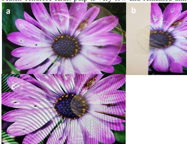
*Figure 8: Films made from mechanically dispersed Kraft pulp, (b) BCTMP, (c) Beaten Kraft pulp fibers. In the case of mechanically dispersed cellulose the water retention increased substantially and formed the most stable suspensions.*
