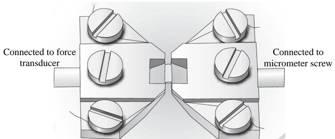
**Figure 2-6: Diagram of segment of uterine artery mounted in wire myograph.**
