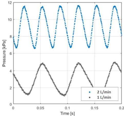
Figure 5. Difference in pressure recorded across the flowmeter using the peristaltic pump flowrate at approximately 1 L/min and 2 L/min.
