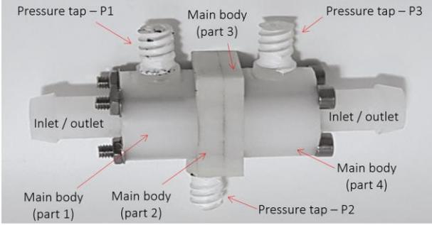
Figure 1. Image of the flowmeter prototype.
