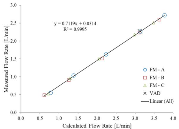
Figure 8. Calculated flowrate from the flowmeter vs the measured flowrate from the mass scale for three similar prototypes.
