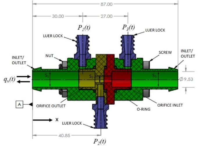
Figure 2. A cross section view of the flowmeter assembly. All units are in millimeters.
