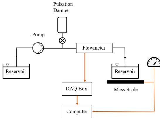
Figure 3. A schematic of the experimental setup.
