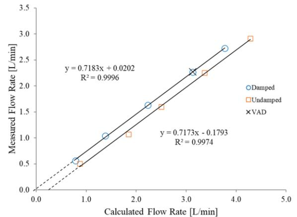
Figure 7. Calculated flowrate from the flowmeter vs the measured flowrate from the mass scale with and without a pulsation damper in series.
