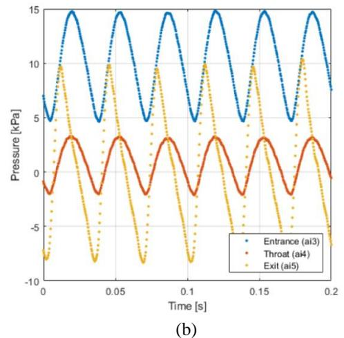
Figure 4. Pressure transducer data collected using the peristaltic pump flowrate at (a) 1 L/min and (b) 2 L/min.
