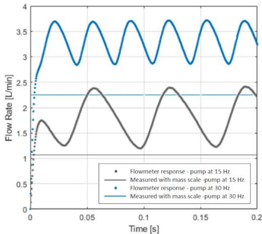
Figure 6. Calculated flowrate from the flowmeter using the peristaltic pump flowrate at approximately 1 L/min and 2 L/min.
