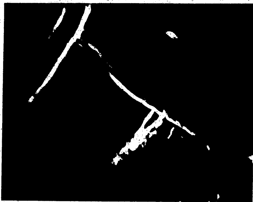
Figure 10. A well developed extrusion and the accompanying cracks or fissures. 5,000X 68,000 cycles fatigued in air.
