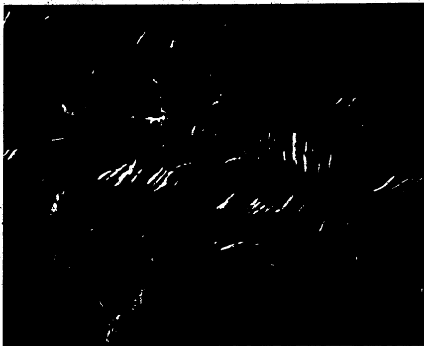
Figure 7. Extrusion formations at 700X fatigued in wet hydrogen. 4,000 cycles.
