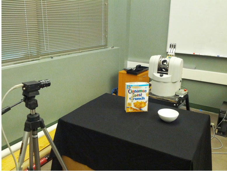
Figure 4.1: Set up for recording videos under normal light using a WAM arm [1] and a Barret hand. The camera is set 120 cm from the base of the robot arm.
