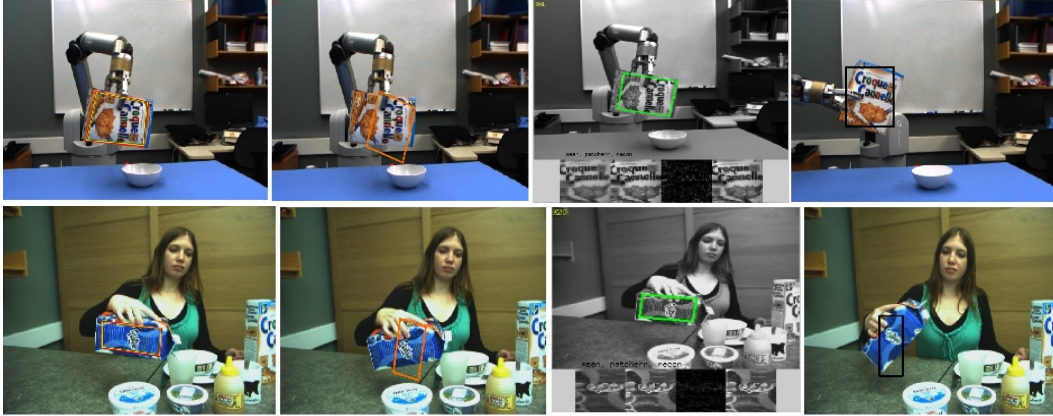
Figure 5.1: L1-APG (orange) [57] and TLD (black) [42] fails to track in plane rotation. Registration based trackers, ESM (red) [9], IC (yellow) [6] and NNIC (cyan) [23] and IVT (green) [67] tracks without considerable drift
