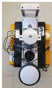
Figure 1: Jackal Unmanned Ground Vehicle (UGV) Robot from Clearpath Robotics
