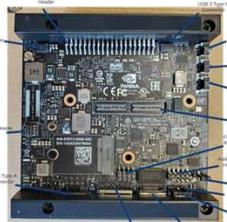
Figure 3: Jetson AGX Xavier single board computer is the upgraded computer implemented in the Jackal for optimization of the AI capabilities of the robot.
