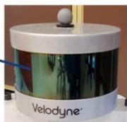
Figure 5: Velodyne Lidar Puck High-Res sensor is a 3D light detection and ranging sensor that uses lasers to ping off objects and return to the source of the laser.
