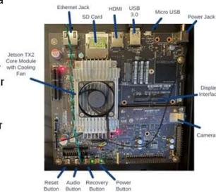
Figure 2: Jetson TX2 single onboard computer is the second computer installed in the Jackal. Most of the software learning that is required to operate the computer took place with this device.
