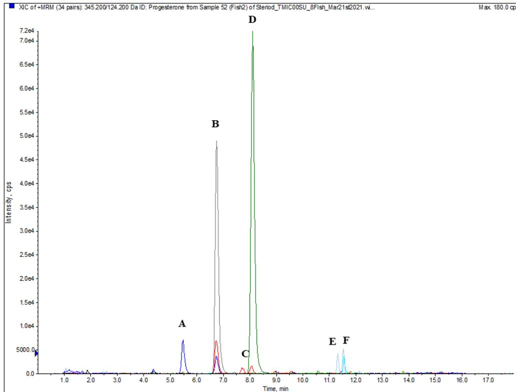
**Figure 3.9 Representative chromatogram from targeted LC-MS/MS analysis of hagfish plasma from a fish without steroid injection. Main peak regions identified are A) Estrone, B) Dehydroepiandrosterone, C) 17-Hydroxyprogesterone, D) d3-Testosterone, and E) Progesterone, and F) Pregnenolone.**
