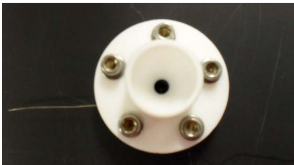
Figure 2.2 Photograph of the O-ring apparatus. A PPF sample is mounted horizontally between a Teflon base plate and a Teflon cell, which has a hole in the bottom and is secured on top of the base plate by five screws. A Viton O-ring placed under the hole is used to seal the solution above the PPF sample. Electric contact to the PPF surface is made using a silver stripe placed on the surface but not exposed to the solution.
