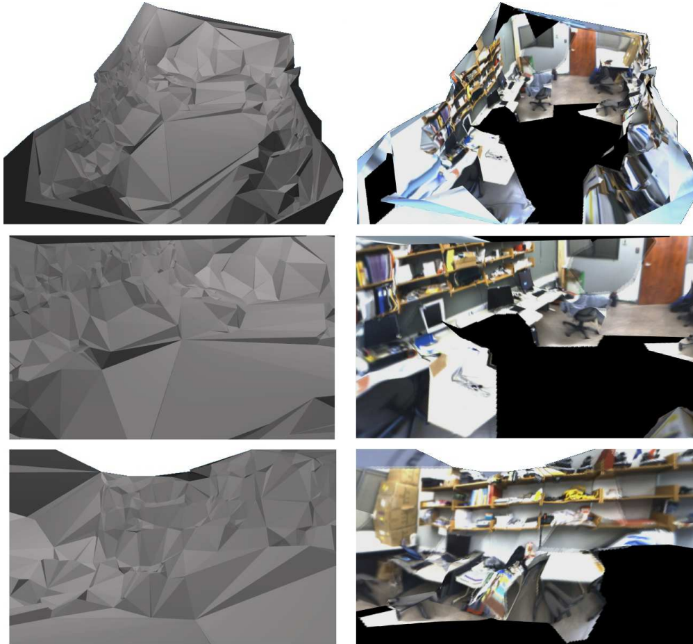
Figure 5.2: A model of the Robotics research laboratory constructed with our system, using smoothing parameter \lambda = 0.3 . Left: Geometry, shaded. Right: Textured rendering, from the same view-points.
