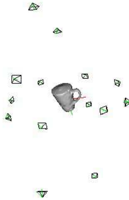
Figure 5.7: View sampling conditions for all the synthetic data experiments. Fourteen camera views are arranged approximately over two rings around our object, one horizontal and one vertical.
