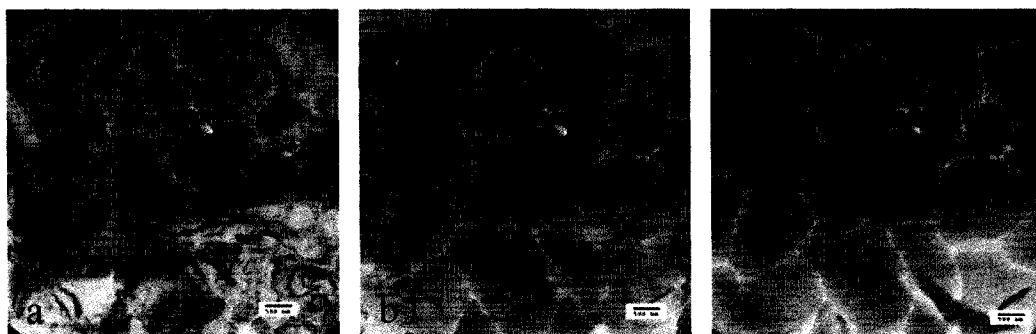
Figure 3.2. Change in morphology observed in bright field images of pentacene films as a result of electron beam damage.
