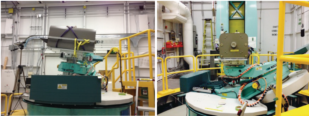
Figure 3.1 The Victoreen 480 free air ionization chamber mounted on the MRT Lift in the SOE-1 hutch on the 05ID-2 beamline for beam stability and quality measurements.
