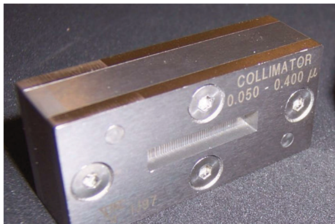
Figure 2.16 The multi-slit collimator at the CLS. The tungsten alloy collimator has 75 50 \mu\text{m} wide slits separated by 400 \mu\text{m} centre-to-centre, and is 8 mm thick. (Image courtesy of BMIT staff.)
