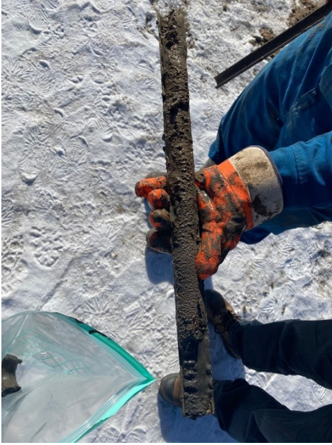
Figure 3-3: Split Spoon Sample (Wet Fine Sand) Collection.
