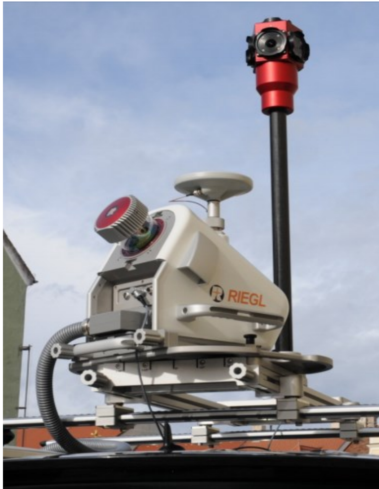
Figure 5 RIEGL VUX-1HA Mobile Laser Scanner
