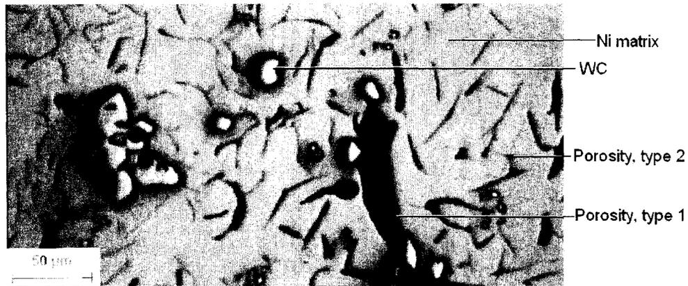
**Figure 4.1: Micrograph of 11.5minute sample from experiment W2.**
