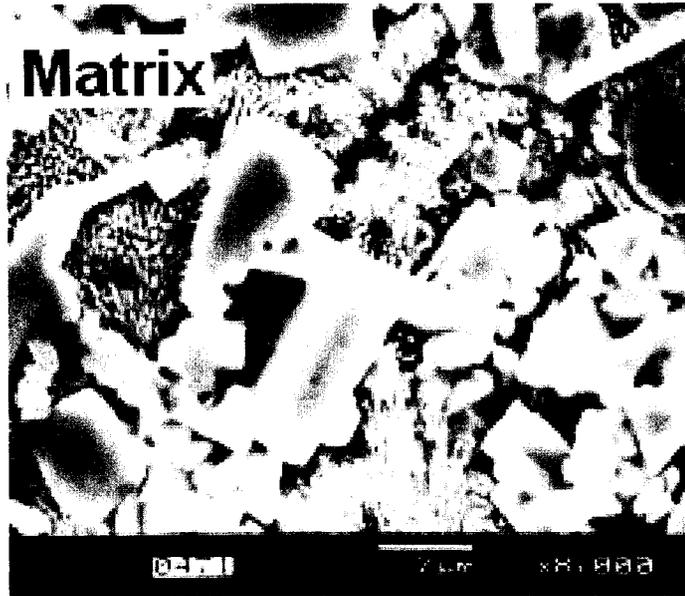
**Figure 2.7: SEM micrograph of the Ni-matrix material from Li et al.<sup>12</sup>**
