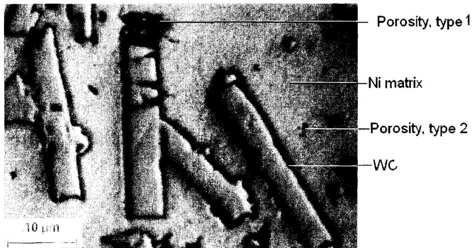
**Figure 4.2: Micrograph of 37minute sample from experiment W2.**
