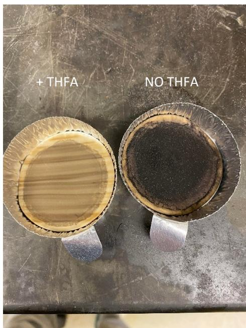
**Figure 18: Insoluble collected from LCO-36-MZ with and without THFA after heating**
