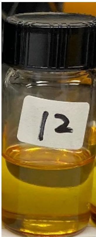
**Figure 26: Visual representation of indene sample after heating at 150 °C with 6 % THFA. The reaction time was 48 hours.**
