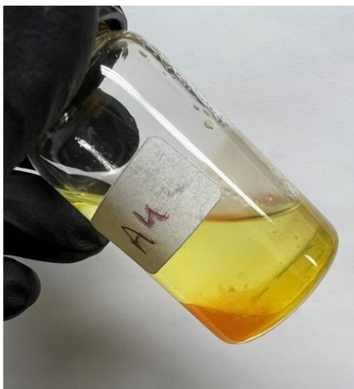
**Figure 48 Visual representation of the aged Indene +THFA mixture after heating at 200 °C.**
