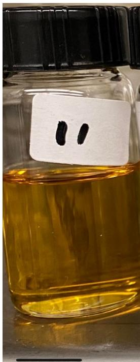
**Figure 24: Visual representation of indene sample after heating at 150 °C with 3 % THFA. The reaction time was 48 hours.**
