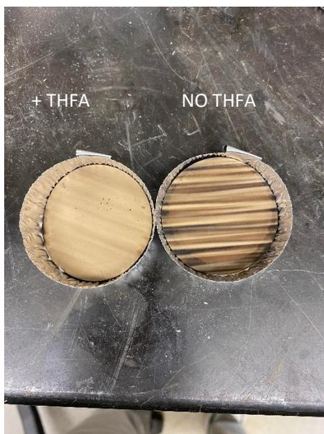
**Figure 16: Insoluble collected from SLCO-43-SZ with and without THFA after heating**
