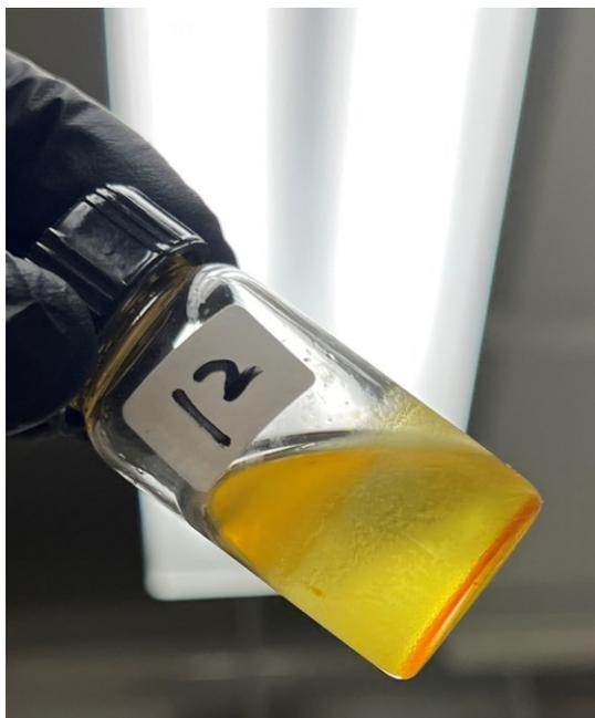
**Figure 27: Visual representation of aged indene sample after heating at 150 °C with 6 % THFA**
