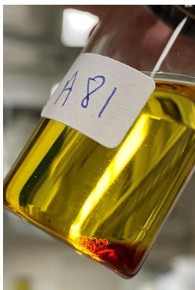
**Figure 63: Visual representation of the indene + ether mixture after heating at 230 °C and 48 hours**
