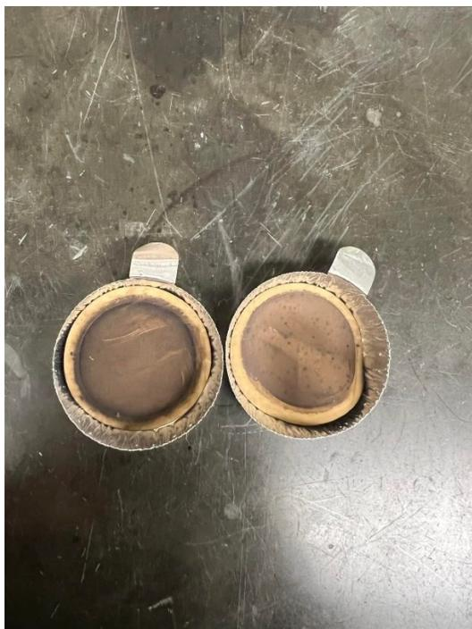
**Figure 19: Insolubles collected from LCO36MZ with 10 wt% THFA without heating**
