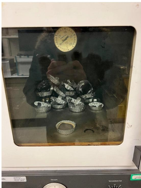
**Figure 12: Visual Representation of the filter paper drying inside the oven.**
