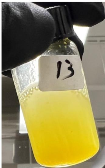
**Figure 23: Visual representation of aged indene sample after heating at 150 °C with no additives. The sample was aged for three months.**
