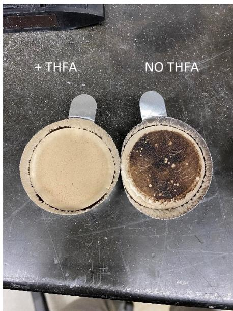
**Figure 15: Insoluble collected from COND-54-NZ with and without THFA after heating**
