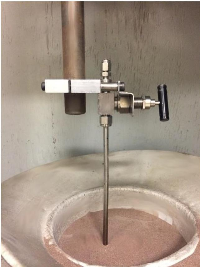
**Figure 11: Visual representation of the micro-batch reactor immersed in the heating sand bath**
