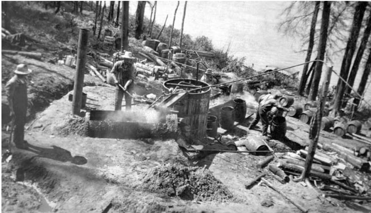
Fig. 26. Robert Fitzsimmons, International Bitumen Company Limited . Unidentified men using early process in liquifying bitumen.
