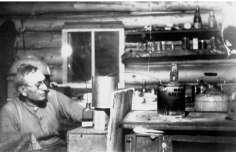
Fig. 17 Daniel Diver, Interior of Shack with Sample of Tar Sands and Extractions, Fort McMurray . Remarks: "Pail on stove holds tar sands, bottle shows oil and a milk like substance. Gas comes from tube at other end. 8 pounds, sand produces 12 ounces, oil; 6000 poundss, sand produce 1 pound bitumin (sic)."
