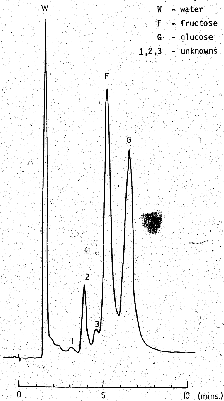
Figure 41. A typical HPLC chromatogram of isomerised product.
