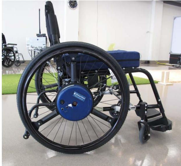
Figure 3- 1 Smart<sup>Wheel</sup> attached to a Quickie manual wheelchair
