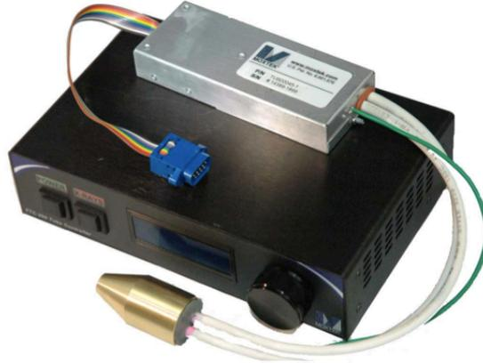
Figure 5.7: The X-ray copper reflection tube (Moxtek) along with the 40 kV power supply and controller [107].
