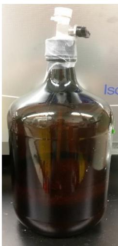
**Figure 3-2.** Toluene purification/storage bottle.
